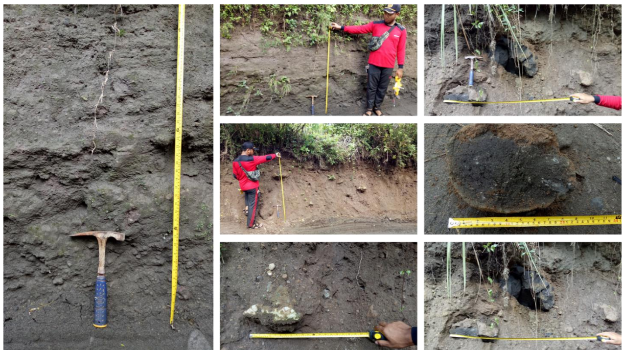
Figure 9 Volcanic sediment outcrop of Kelud Muda (Qvk) is located in the southeast slope of Mount Kelud. This agglomerate-composed volcanic sand layer was found in resident well at 5-13 m depth.
